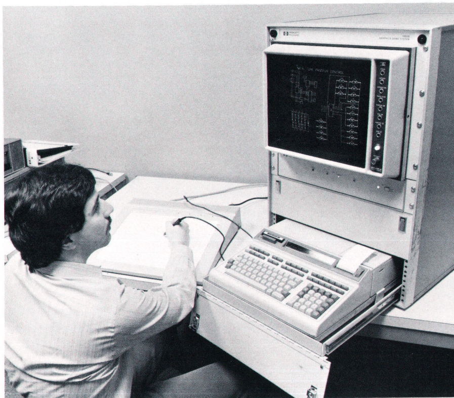
Fig. 1. The combination of a 9111T Graphics Tablet, a 1350S Display System and a controller such as the 9825 provides powerful interactive graphics in an inexpensive workstation.
